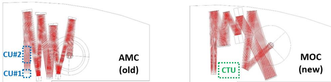
Figure 3. Comparison between old and new MAORY PFRO design: the impact on CTU position and volume.
