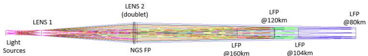
Figure 6. Zemax model of the Focusing Optical System (FOS).
