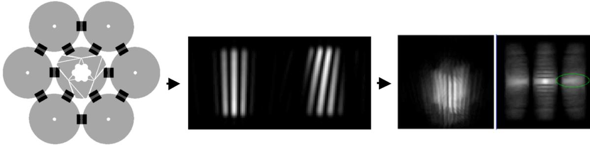
Figure 3: Left: The GMT pupil overlaid with 12 1.5-m square apertures at the segment boundaries. Center: Simulated fringes from one subaperture showing in phase (left) and a 10-micron phase shift (right). The dispersion direction is vertical. Right: A simulated dispersed fringe image and its FFT. The vertical displacement of the circled peak is a function of the tilt of the fringes and thus a measure of the phase error.
