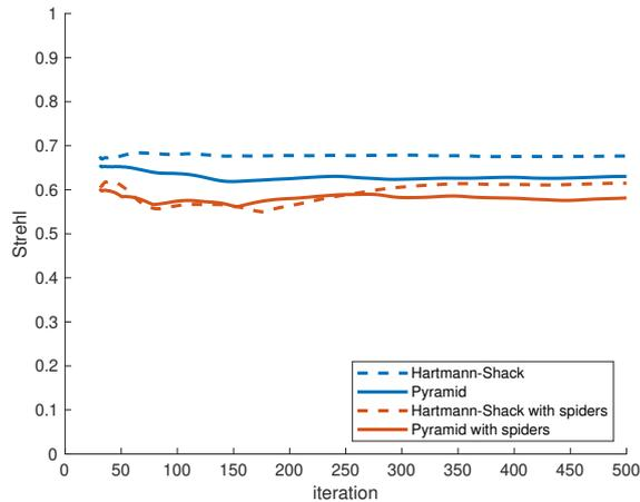
Figure 4. Strehl evaluation of linearized roof and Hartmann-Shack wavefront sensor in tomographic mode, with and without spider legs.
