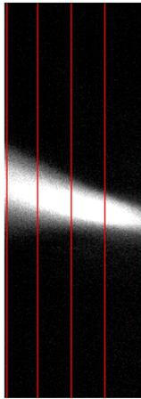
Figure 4. Selected region of the plume; the light distribution along the red lines has been selected for further analysis.
