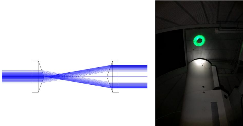
Figure 2. Zemax layout of the positive and the negative axicon in the LGS launch system and the ring-shaped generation with the axicon at the OGS dome.
