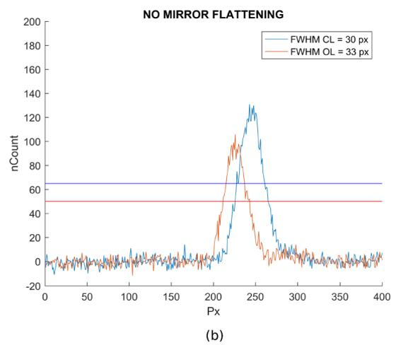
Figure 6. Laser intensity distribution corresponding to the most focused point the laser plume (last red line in Figure 4); in red open-loop operation, in blue, close-loop operation with (a) and without (b) performing the DM flattening
