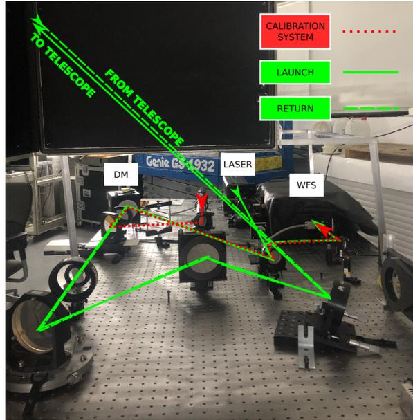
Figure 1. The light from the Verdi laser follows the solid line through the optical elements, the deformable mirror and the folded mirrors which inject the laser beam to the telescope tube; on the return path (dashed line), the light coming from the sky follows the exact same optical path until the 50/50 beam splitter which divides the beam and leads it to the WFS. In red, the calibration system described later in this chapter.
