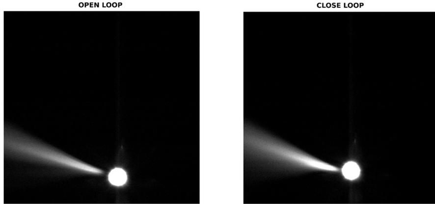
Figure 3. Scoring camera images of the laser plume before and after closing the AO loop with Arcturus as NGS, also in the image. Notice the increase in brightness when the laser wavefront is being pre-compensated.
