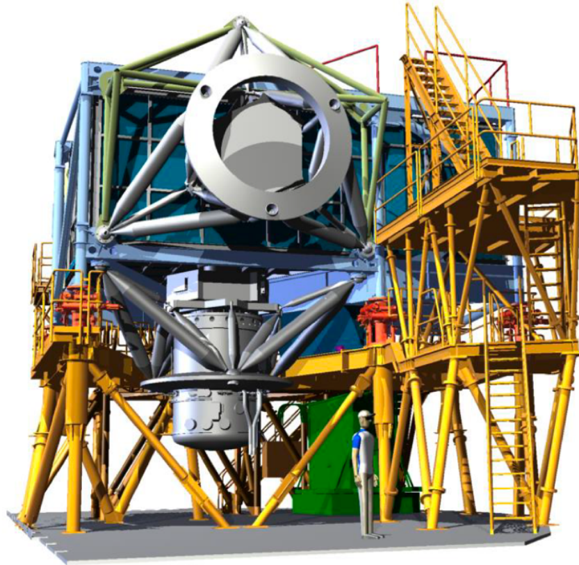
Figure 1: NFIRAOS (in blue) as it would appear from the TMT Nasmyth platform. The client instrument IRIS (grey) is shown below NFIRAOS. The NFIRAOS electronics enclosure is shown in green.
