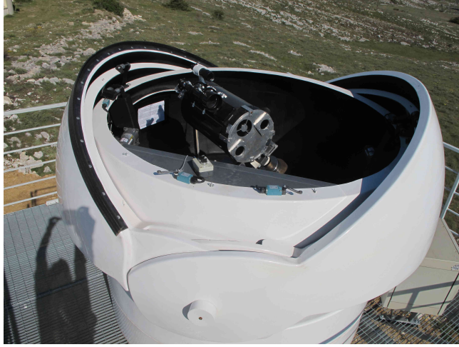
Figure 2. The GDIMM instrument inside its 7 ft AllSky dome which is installed on a platform at 4m above ground level (left of Fig.1).
