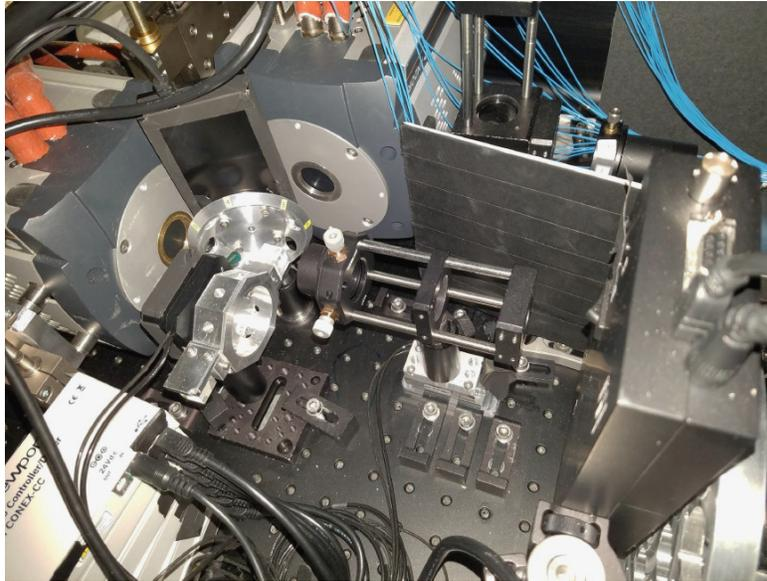
Figure 2. Picture of the VAMPIRES module inside SCEXAO. The two cameras are located at the top left, with the differential filter wheel in between, and the beamsplitter cube wheel in front of it.
