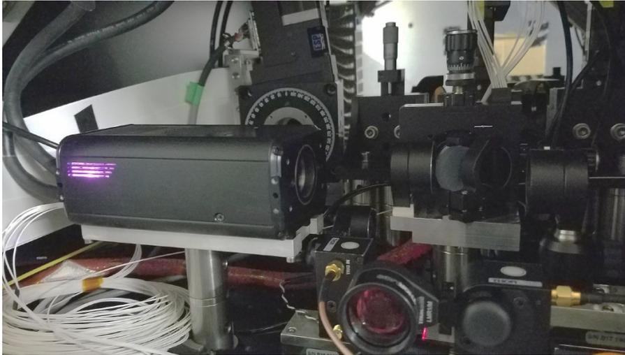
Figure 7. Picture of the internal C-RED2 camera used for the current fast IR polarization mode.
