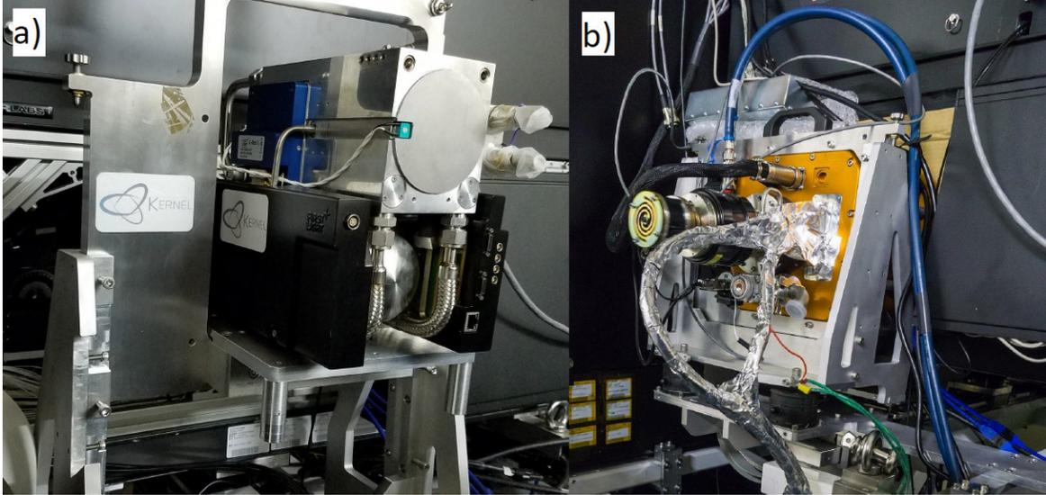
Figure 9. Two fast IR photon-counting camera tested on SCEXAO. a) The Kernel camera, a C-RED ONE from First Light Imaging. b) IfA's custom SAPHIRA camera.
