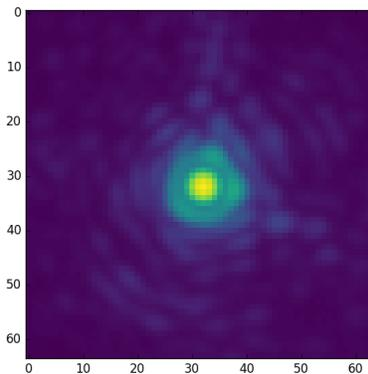
Figure 1. High-Strehl on-sky images taken with VAMPIRES. This image was created from a cube of images taken at high frequency, recentered to remove jitter, and co-added.
