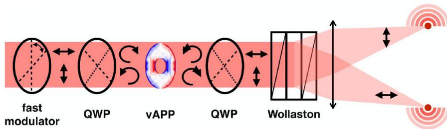
Figure 10. Principle of a polarized vAPP.
