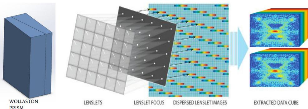
Figure 4. Principle of the spectro-polarimetric mode with CHARIS. The Wollaston splits the two polarizations close to a pupil plane at the entrance of CHARIS, then after entering the Dewar, the light in the focal plane is sampled by a matrix of micro-lenses and an array of pinholes, and dispersed by a prism. The final cube is extracted from the raw image. Each polarization occupy half the normal field of view of CHARIS, i.e.  $2 \times 1$  arcsec.
