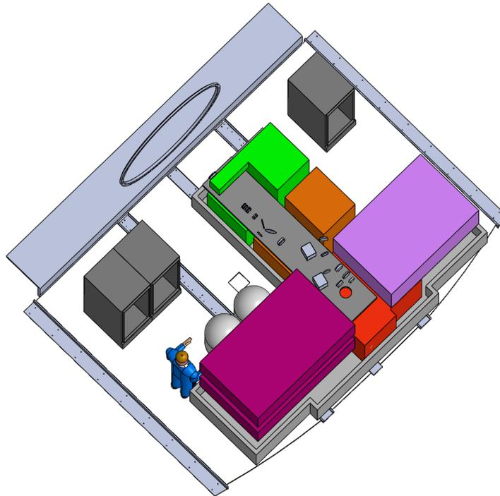
Figure 7. Current snapshot of the overall MAVIS mechanical layout on the AOF Nasmyth platform. The AOM PFR is the gray long optical table in the middle, surrounded by the LGS WFS space (orange), the Calibration unit (green), the NGS WFS (red), the imager (violet, right) and the spectrograph (purple, left). Cabinets are in dark grey. The interface to the AOF adaptor rotator is toward the top left.
