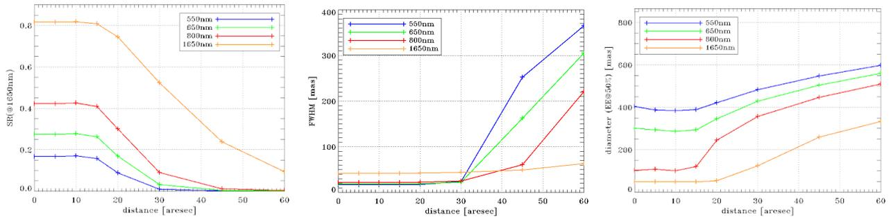
Figure 2. Performance expressed as Strehl ratio (SR), Full-Width at Half Maximum (FWHM) and diameter for 50% of EE, of MAVIS AOM (AO errors only) for a good NGS asterism (bright and near the science field, 20" off-centre).
