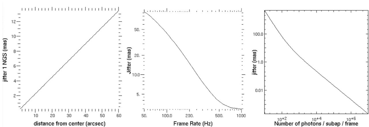
Figure 4. Jitter from tomographic (left), temporal/windshake (middle) or noise (right) error. The tomographic error is given for 1 NGS only.
