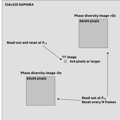
Figure 9. Conceptual layout of the NGS WFS chip occupation, including TT star image, together with phase diversity defocused image for truth sensing.
