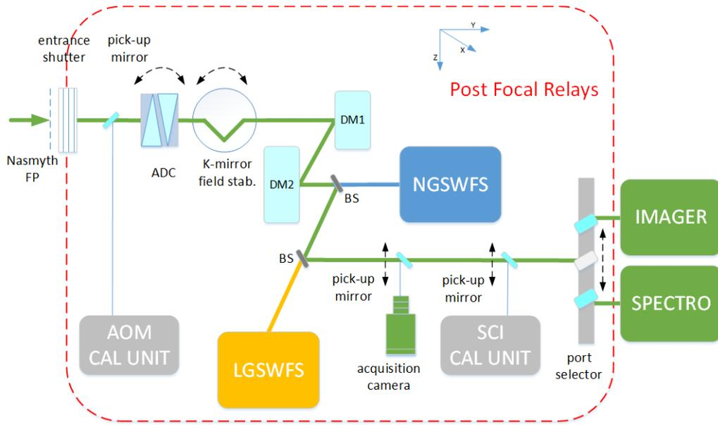
Figure 6. An illustration of the MAVIS conceptual design, showing the AOM Post Focal Relays, NGS WFS and LGS WFS sub-modules, and the Imager, Spectrograph and Calibration Unit modules.
