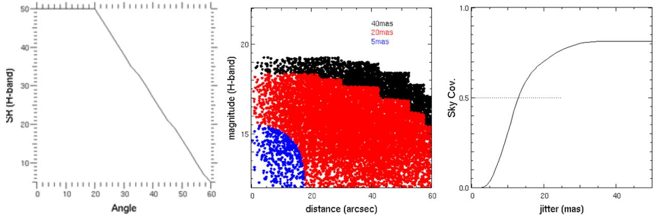
Figure 5. Figure 5. Left: Assumed SR in H band in function of off-axis angle. Middle: Jitter as a function of the average distance of the NGSs and their total magnitude. Right: Sky coverage jitter curve.
