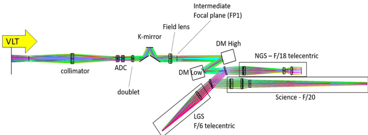
Figure 8. Optical layout of the MAVIS baseline transmissive PFR design. All powered optics are on-axis. Note that this optical layout will be reworked soon, e.g. the exact F/ ratios for NGS and LGS channels will be optimised.
