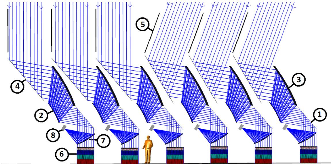
Figure 9. Using the beam expander optics to receive a signal for atmospheric correction by inserting a dichroic mirror (7) between the laser block (5) and the beam expander optics.
