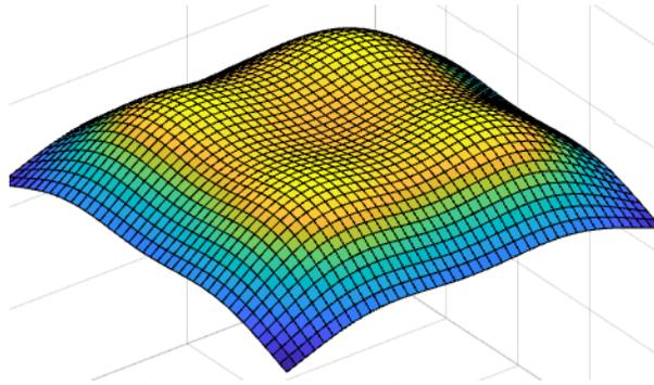
Figure 1 An example lobed beam profile created by summing the intensity of four offset Gaussian beams.
