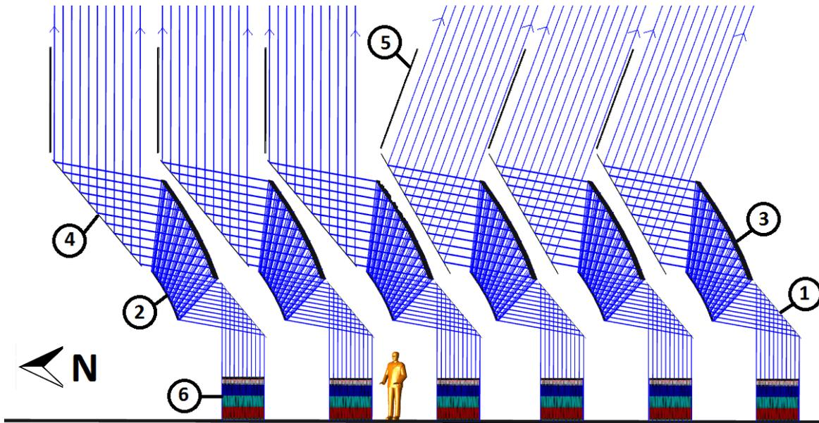
Figure 7. Six projector units, each with a fixed laser block and 2x beam expander where light passes through a focus, seen from the west. The 3 steering flats on the left direct the beams to the zenith, those on the right to 65° elevation. Mirror 1 is a segmented adaptive fold flat. Mirrors 2 and 3 constitute a beam expander. Mirror 4 is a steering flat. 5 are hinged roof hatches. 6 are laser blocks.
