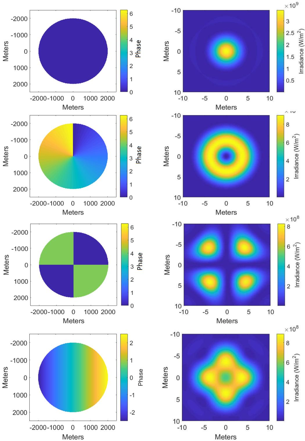
Figure 2 Beam aperture phase plots (left) and their corresponding point spread functions at the spacecraft sail (right). Note that the color scales on the PSF plots are not the same. The bottom PSF plot is the sum of four PSFs each generated by a phase distribution rotated 0, 90, 180, 270 degrees respectively from the one shown on the bottom left.
