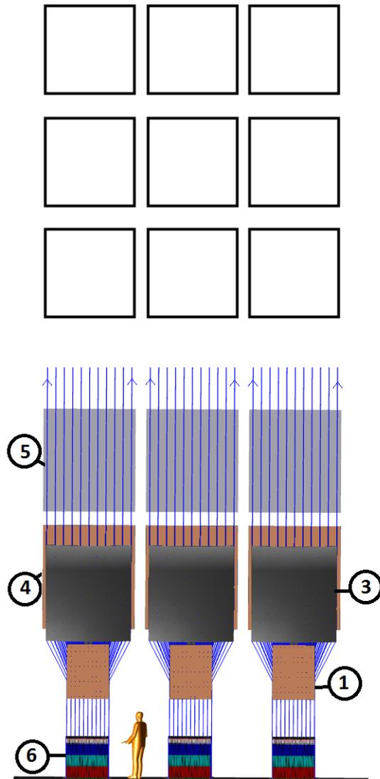
Figure 8. Top: the beam pattern for a 3x3 group (zenith pointing) as seen from the spacecraft. Bottom: a view of the beam expanders looking south.
