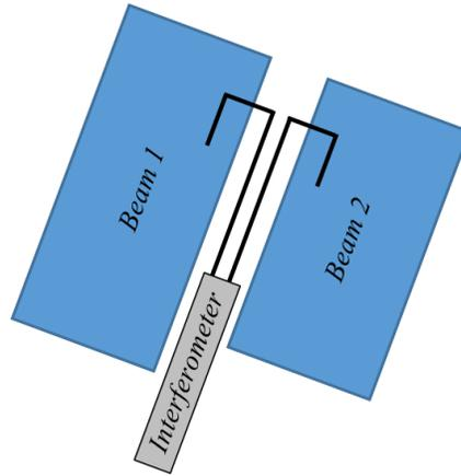
Figure 4. A schematic diagram showing fiber optics sampling two laser beams and combining the samples to measure the phase difference between them.
