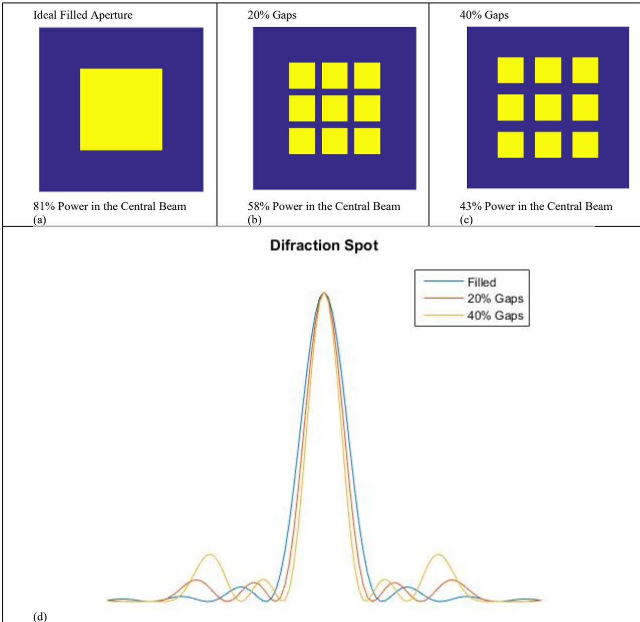
Figure 6. (a) An ideal filled aperture. (b) An aperture with 20% spacing between subapertures. (c) An aperture with 40% spacing between subapertures. (d) A plot of the irradiance cross sections of the diffraction patterns of the apertures shown in (a), (b), and (c).
