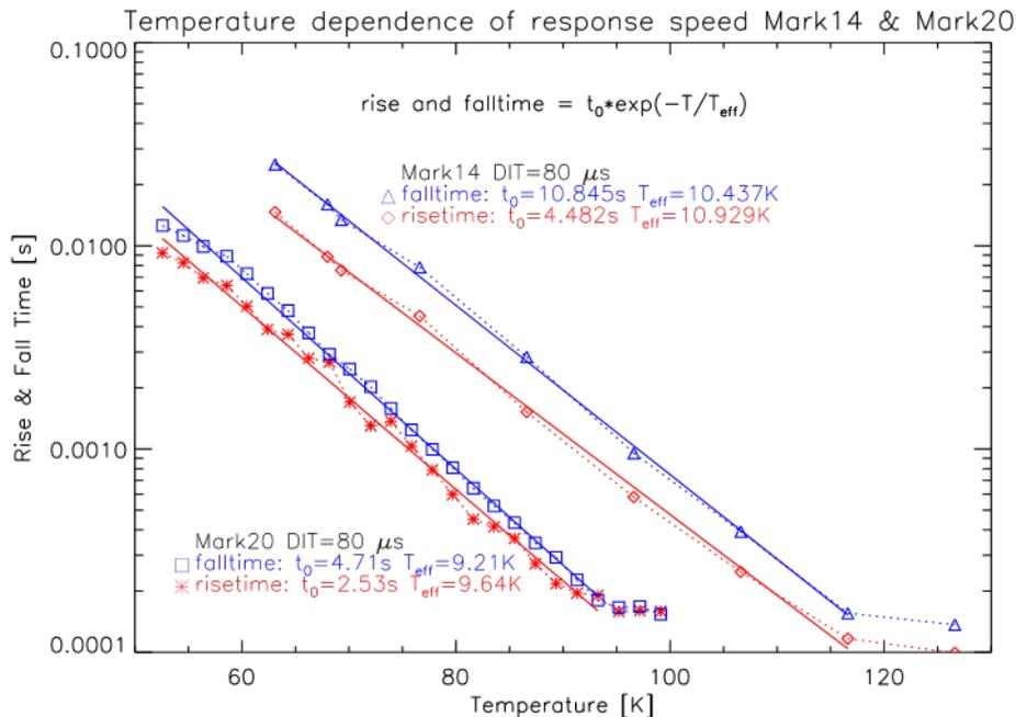
Figure 5. Comparison of rise and fall times of Mark14 and mark 20 arrays as a function of temperature.
