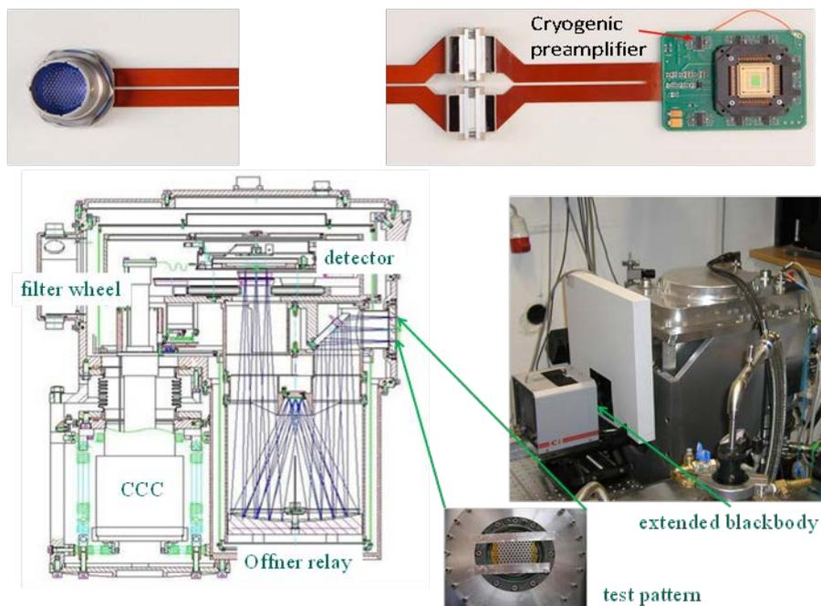
Figure 2 Top detector in LCC socket on detector board with cryogenic preamplifiers and flexible boards, connectors for radiation shield and hermetic connector. Bottom: cryogenic camera with Offner relay Offner and two filter wheels. Right: extended blackbody and test pattern on entrance window in image plane of detector.
