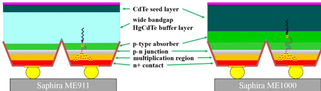
Figure 1. Left: Mark3 MOVPE diode design with wide bandgap buffer layer limiting short wavelength response to  $\lambda > 1.3 \mu\text{m}$ . Right: Mark14 MOVPE diode design without wide bandgap buffer layer sensitive from 0.8 to 2.5  $\mu\text{m}$ .
