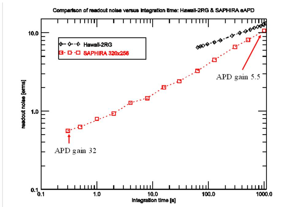
Figure 4 Comparison of readout noise of Hawaii-2RG array and SAPHIRA Mark14 array as function of detector integration time at optimum APD gain.
