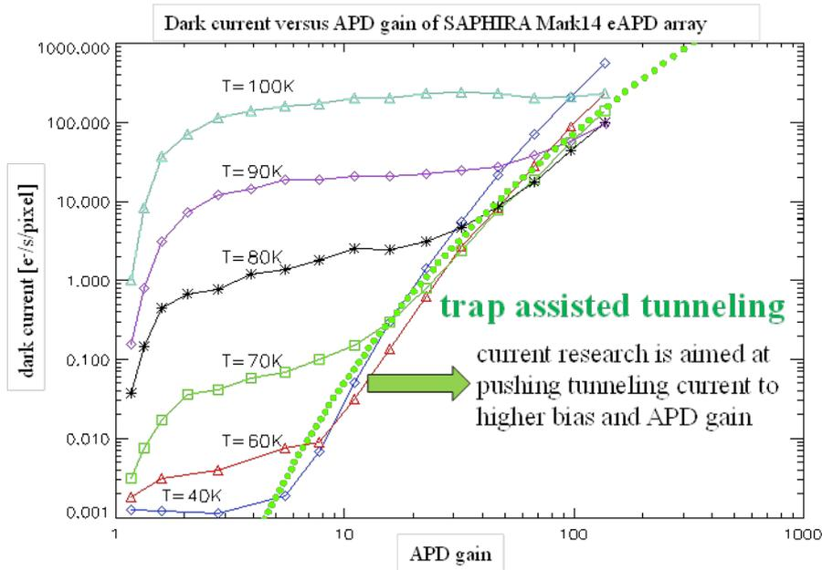
Figure 3 Dark current as a function of APD gain for different detector temperatures. At a detector temperature of T=40K and low APD gain dark current is 1E-3 electrons/s/pixel. At high APD gain dark current is dominated by temperature independent trap-assisted tunneling. Current research is aimed at reducing trap assisted tunneling at higher APD gain.
