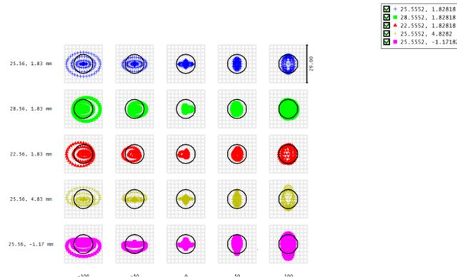
Figure 5. defocus analysis with a simple objective with different locations in the reference focal plane for the beacons.
