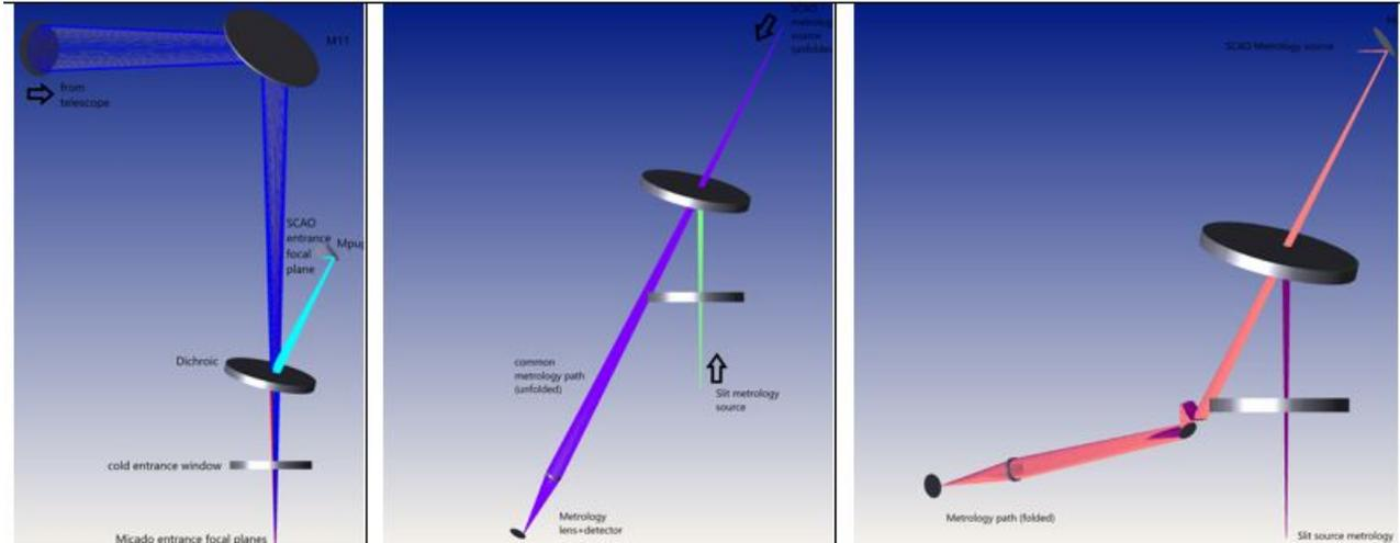
Figure 3. Zemax simplified simulation of the different paths. Left: Paths from the telescopes to SCAO and Cryostat. Middle: Unfolded path from the SCAO and Cryostat focal planes to the metrology camera. Right: Some more realistic folding to adapt to the required space constraints.
