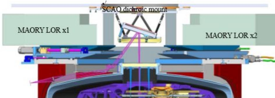
Figure 4. Preliminary Opto-Mechanical layout for the metrology system. It would slide under the Green Donut structure while staying into a room temperature environment.
