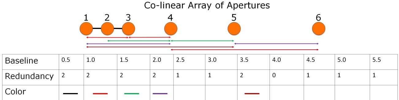
Figure 3. Example N=6 RSC geometry. The apertures are spaced by a half unit for simplicity.
