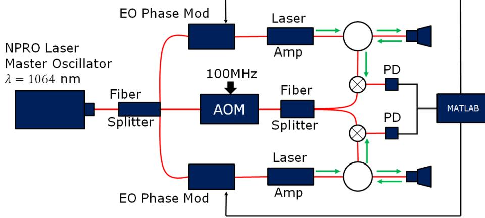
Figure 1. Phase jitter measurement and correction experiment. The LO is frequency shifted by 100 MHz. The MATLAB processing may be replaced by an FPGA depending on the feedback loop requirements.
