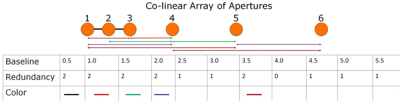
Figure 3. Example N=6 RSC geometry. The apertures are spaced by a half unit for simplicity.
