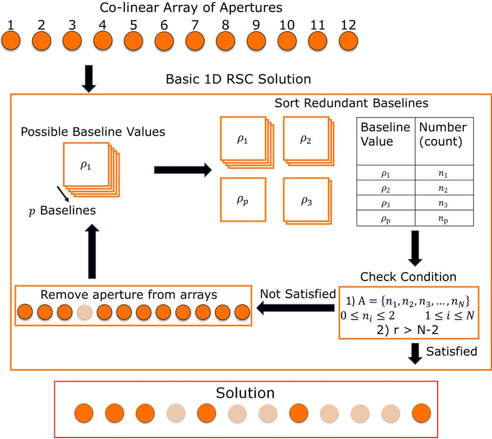
Figure 2. Example RSC algorithm. The circles are the laser launch sub-aperture and the transparent circles are the apertures not considered in the final solution to satisfy the redundancy requirements. The process began with 12 apertures and the solution only left 6 apertures to be co-phased.
