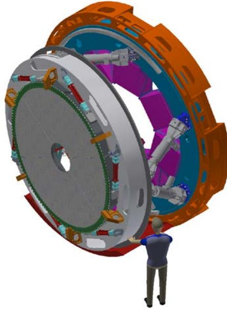
Figure 1: M4 Unit: the orange and blue structure is the Nasmyth Switcher. It includes as well the electronics cabinets in purple. The Adaptive mirror in dark grey (left part of the sketch) is attached to its cell (in light grey) by the lateral and axial supports. The mirror and the cell are attached to the Nasmyth switcher with the hexapod.
