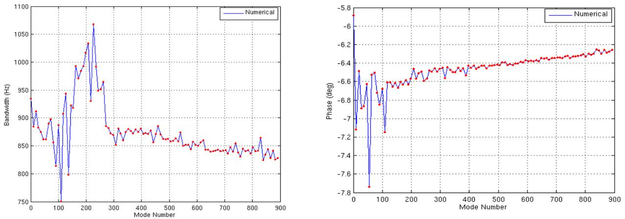
Figure 3: Left: M4 mirror bandwidth versus modal shape command; closed loop transfer function identified on M4 model. Right: M4 mirror maximum phase lag within the bandwidth [0 - 40] Hz for each modal command
