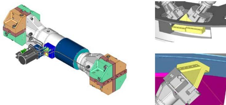
Figure 6: Design of one hexapod actuator and wedges used to fix the actuators to the two opposite structures. The flexible joints are represented by the brown/green structure on the two sides of the actuator, the central part includes the encoder, the gearset, the roller screw and axial bearing
