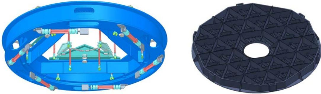
Figure 2: The M4 mirror Cell – shown on the left picture- is a three meters diameter aluminum structure with axial and lateral supports to handle the Silicon carbide reference body – shown on the right picture - as a standard optical mirror.
