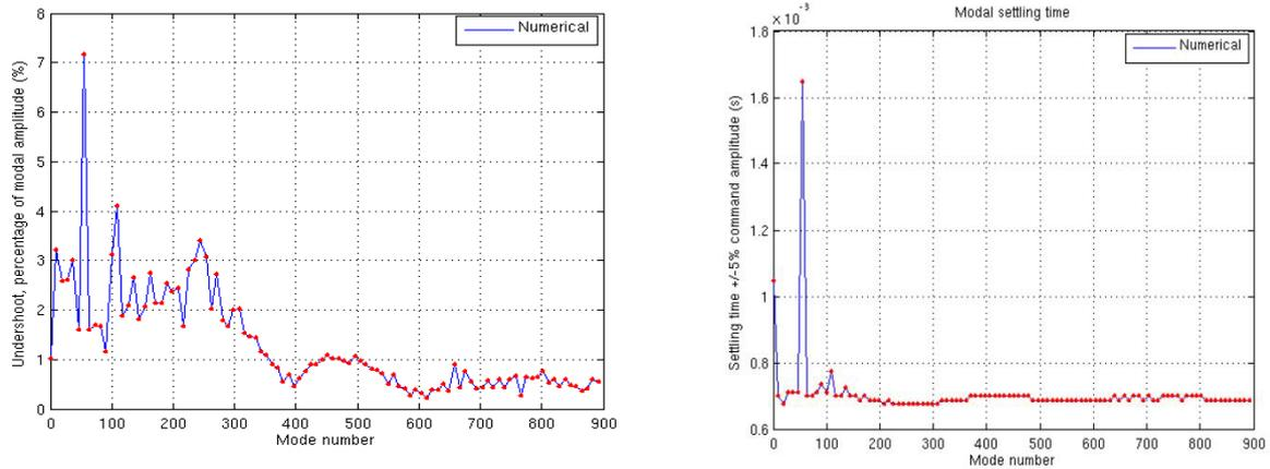
Figure 4: Left: undershoot versus modal command. Right: M4 mirror modal step response settling time. Mode 60 shows a longer settling time because the first cycle of the damped oscillation exceeds the 5% range.
