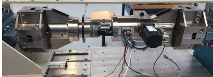
Figure 10: hexapod leg prototype on the test bench
