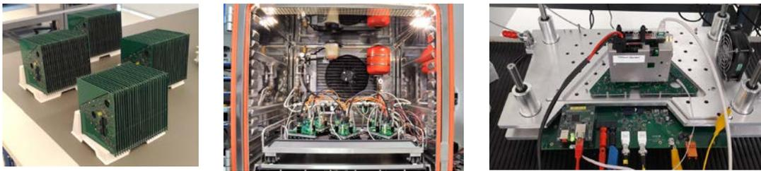
Figure 8: on the left, the driver boards for bricks of type A and B. In the center, the setup for the burn-in tests and on the right the calibration of the driver boards
