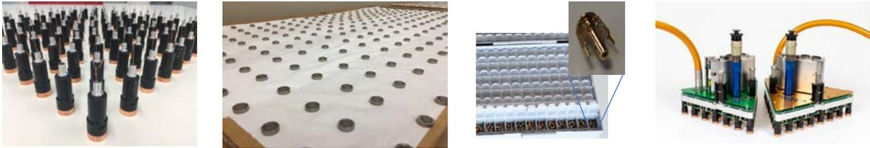
Figure 7: From left to right: voice coil motors ready to be integrated into the bricks, permanent magnets with their Zerodur puck ready to be bonded on the mirror shells, capacitive sensor contacts 60% ready for integration and two bricks integrated and functionally tested.
