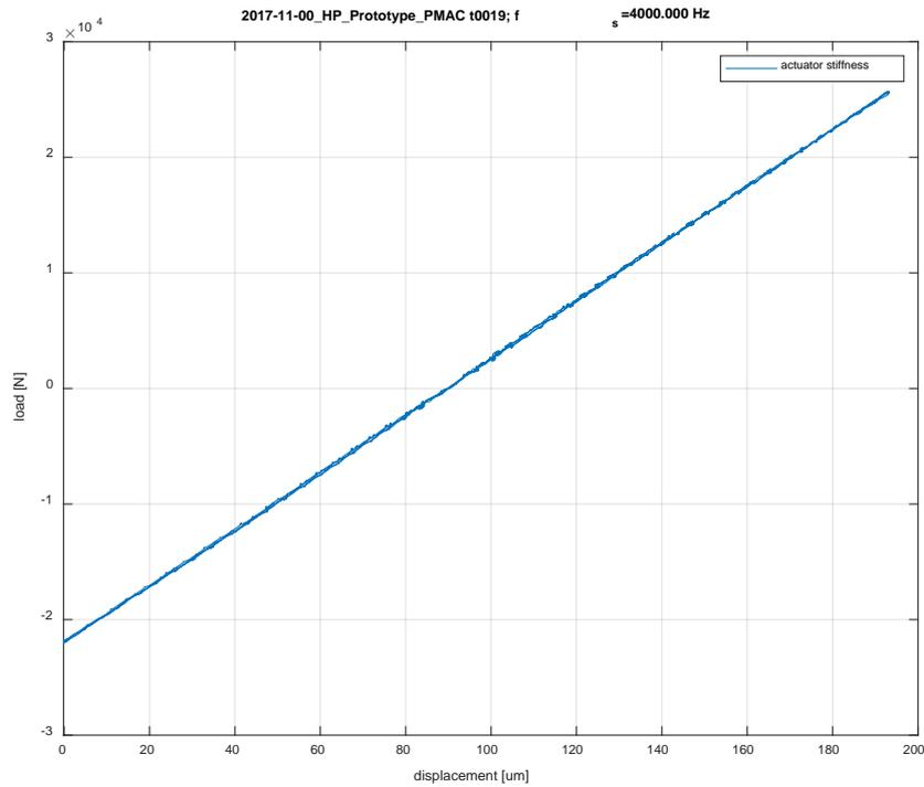
Figure 12: The stiffness of the prototype has been verified experimentally. The stiffness is 246.9 N/micron and the hysteresis is lower than 1 micron.
