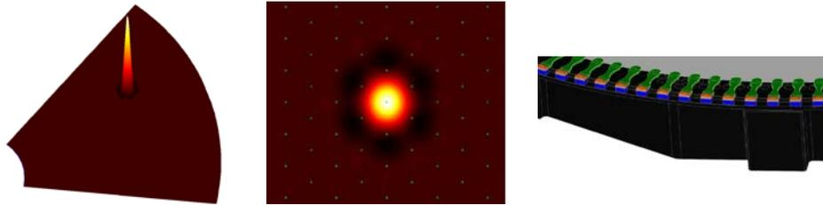
Figure 5: Left and central image: Influence function obtained from the FEA model including the membranes restraining the shells laterally; right image: membranes design
