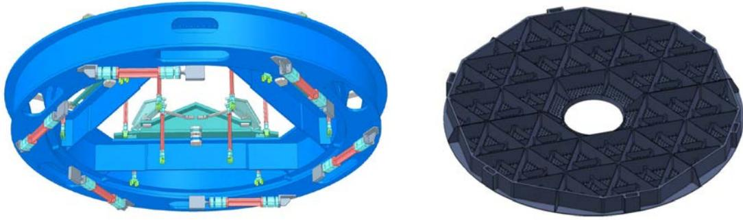
Figure 2: The M4 mirror Cell – shown on the left picture- is a three meters diameter aluminum structure with axial and lateral supports to handle the Silicon carbide reference body – shown on the right picture - as a standard optical mirror.
