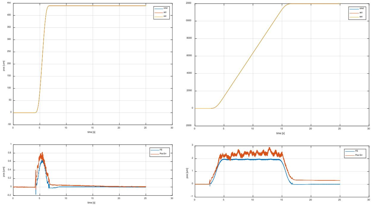
Figure 11: Performance of the actuators for two different steps sizes: on the left for a step of 0.44mm and on the right for a step size of 2 mm. In both case the accuracy obtained is ten times better than the requirements
