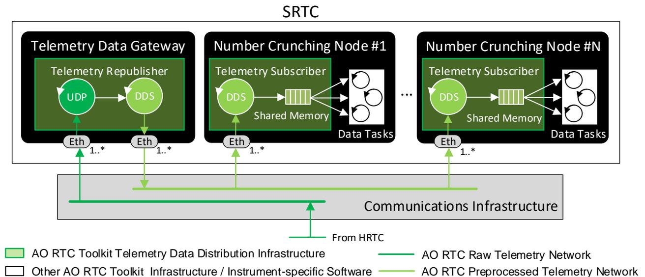
Figure 2. Standardized SRTC telemetry data flow and related computing nodes and software components.
