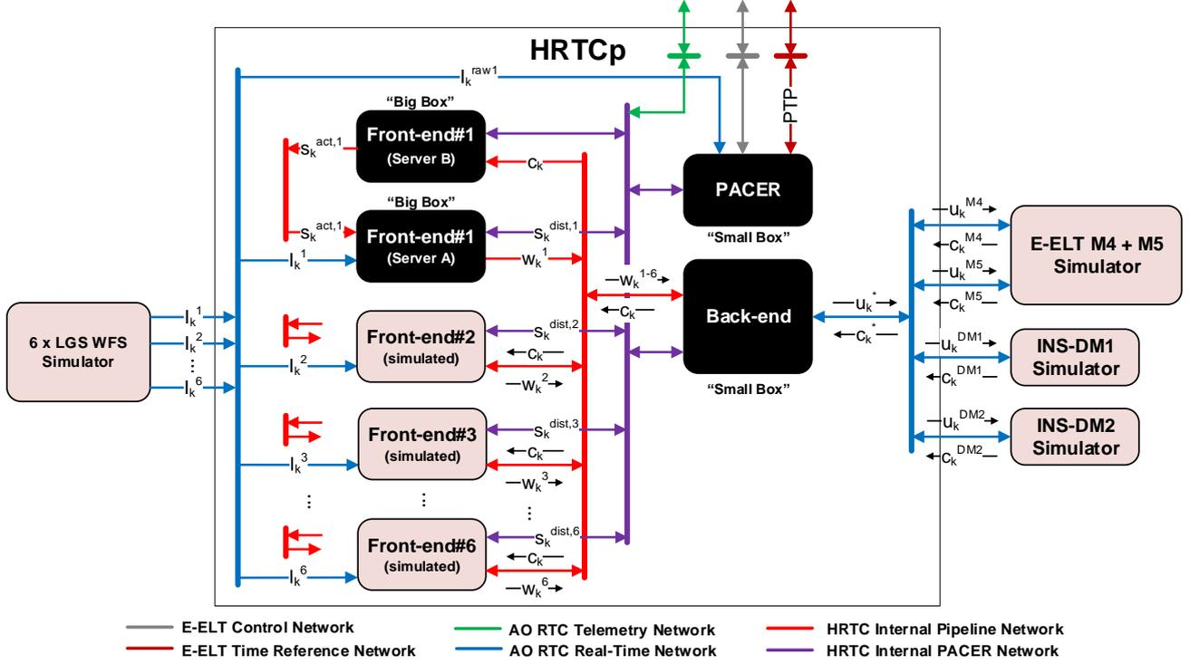
Figure 4. HRTC Prototype topology and main data paths. The thin connecting lines indicate individual network links, whereas the thick ones represent aggregate data paths internal to the network switch.
