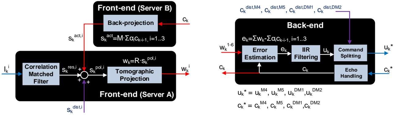
Figure 5. Detail of the HRTC prototype Front-end (left) and Back-end (right) computations. Vectors  $s_k^{res,i}$ ,  $s_k^{act,i}$ ,  $s_k^{dist,i}$  and  $s_k^{pol}$  have size 9,332, whereas the dimension of vectors  $w_k^i$ ,  $c_k$ ,  $u_k$  and  $e_k$  is 6,316.
