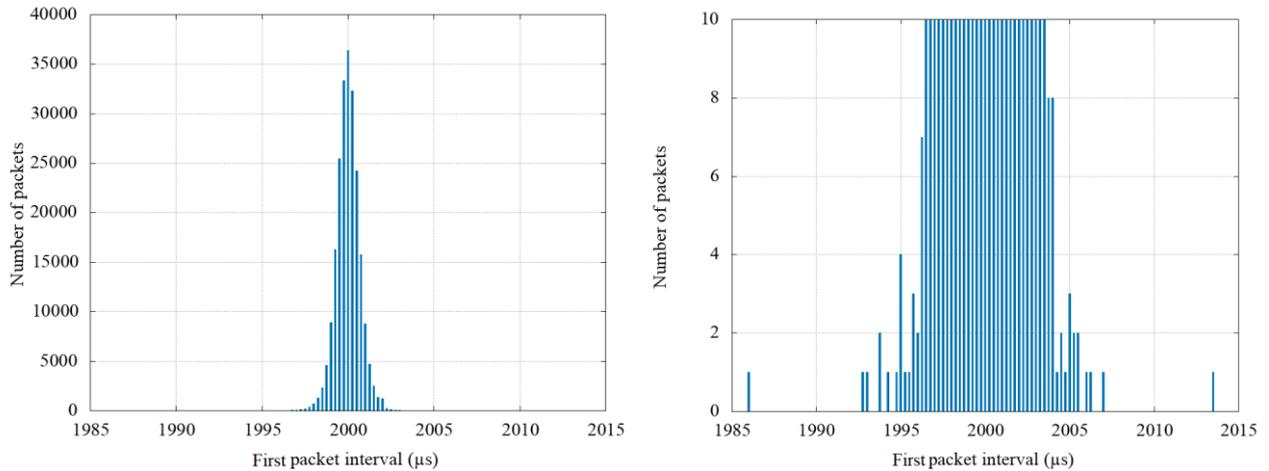
Figure 8. Results from packet transmission test. Left: histogram of the observed interval between the first packet of successive packet trains transmitted with 2 ms period. Right: magnification of the above.
