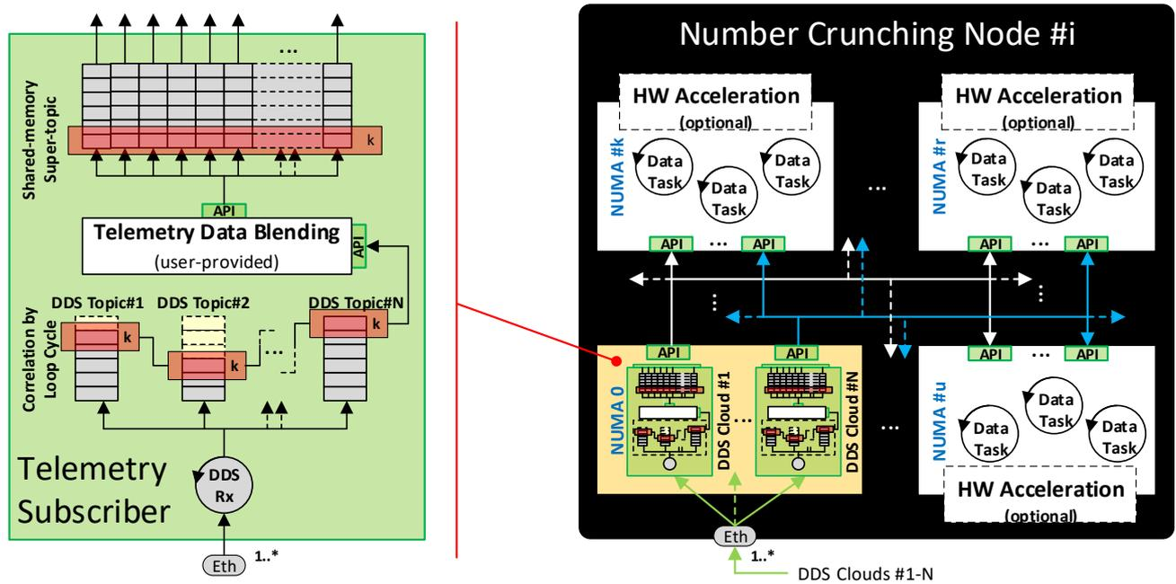
Figure 3. Telemetry subscriber (left) and deployment per node and data cloud (right).
