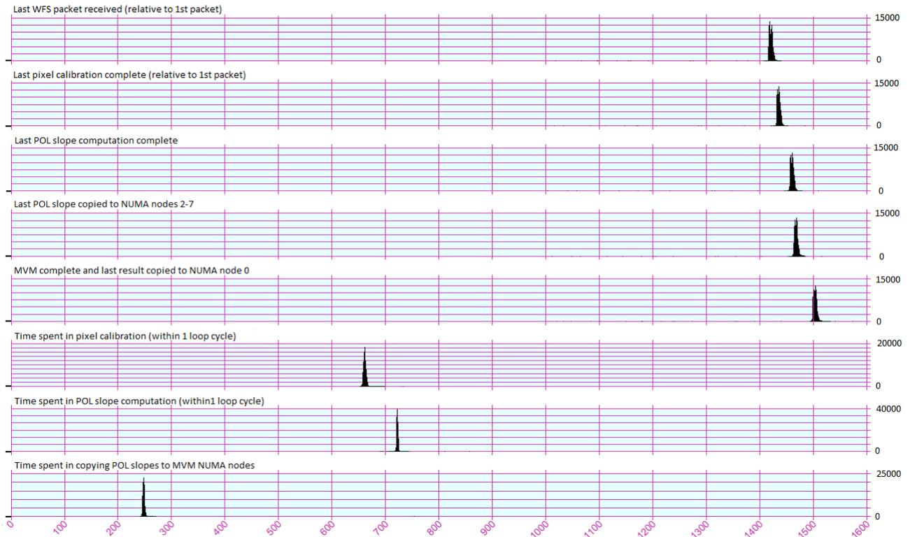
Figure 7. Timing results from the main computations in Front-end Server A. Upper five graphs: histograms of the observed duration of the various Front-end computing steps wrt. the first WFS packet received. Bottom three graphs: histograms of the cumulative time spent in the execution of key computing steps within one loop cycle.
