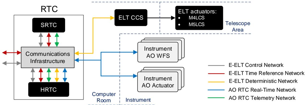
Figure 1. Main functional blocks and communication channels in the ELT RTC.
