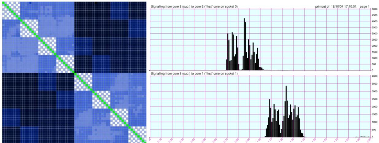
Figure 6. AMD EPYC 7501 inter-core latency map (left) and time to signal 56 threads in remote NUMA nodes (right). Left: green (same core, latency not defined), white (80 ns), medium blue (425 ns), dark blue (1,150 ns). Right, upper graph: signaling between cores in the same NUMA node. Right bottom graph: signaling between cores in different NUMA nodes. The CPU core numbering for the left and right figures follows the AMD and Dell schemes<sup>3</sup> respectively.
