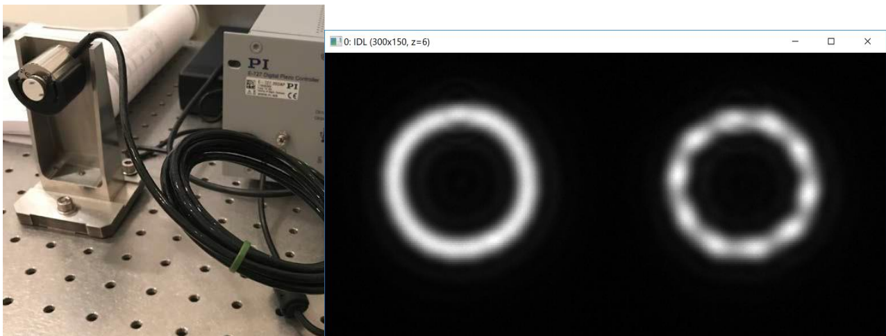
Figure 8: [left] Pyramid Modulator Unit for SCAO, prototyped at LAM. The PI component has been run at ambient temperature at 500 and 1000Hz, with a modulation radius of 5 diffraction sizes. [right] the signal averaged on a 2ms / 1ms exposure time. The discretization of the modulation signal at 10kHz is only visible on the 1000Hz case.
