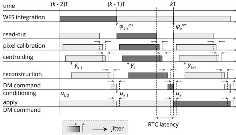
Figure 1. Two frame delay AO loop chronogram showing the overlapping computation times of the pipelined RTC operations. The jitter on the RTC latency is shown as the varying end times for each computation step which results in an overall jitter on the time the DM command is applied. The parameter  $k$  designates the time step,  $\phi^{res}$  is the residual wavefront phase,  $y$  is the wavefront gradient vector, and  $u$  is the DM command vector.
