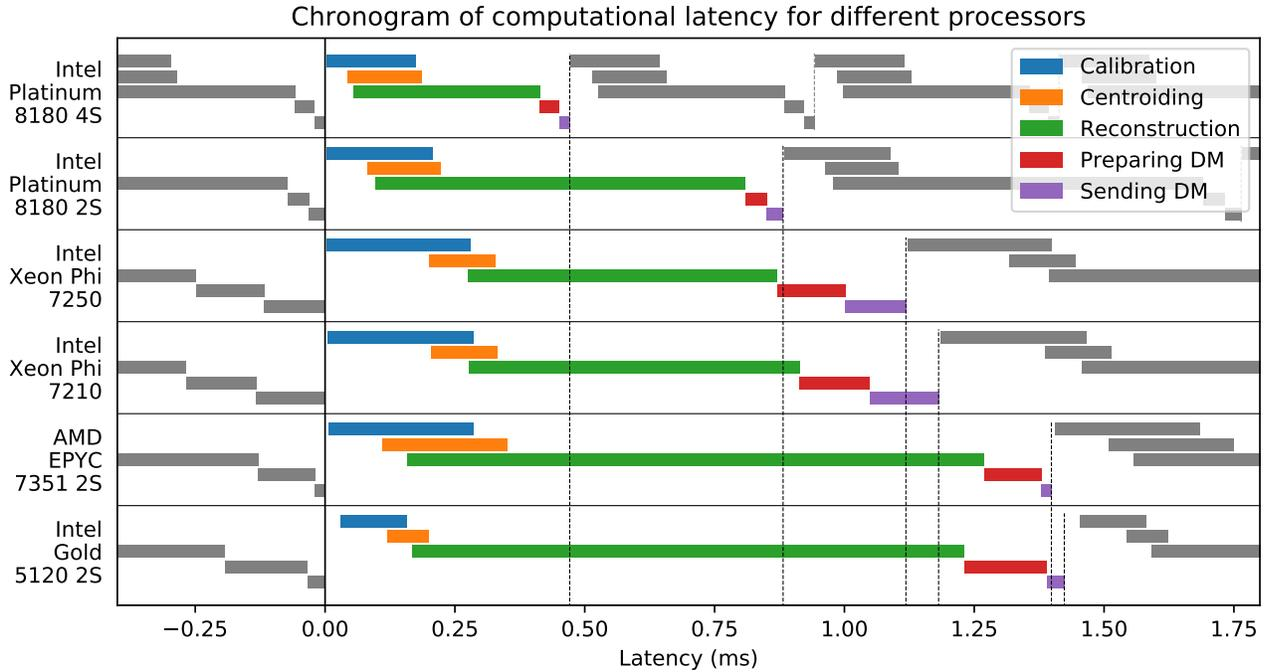
Figure 6. A comparison of the computational latency for different hardware platforms.
