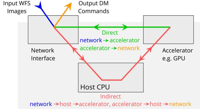
Figure 2. A comparison of the standard indirect data transfer through the host CPU and the more efficient direct to accelerator transfer scheme. A downside to the latter is that it currently involves non-portable software and the use of proprietary libraries.
