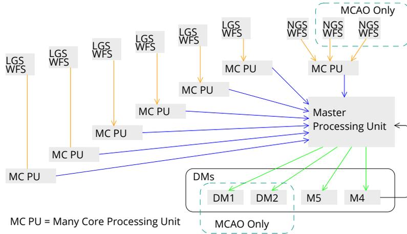
Figure 4. The proposed architecture for the MCAO and LTAO multi node RTC. The 6 LGS WFSs are each processed by a single many-core node. The NGS are all processed on the same node, three for MAORY and one for HARMONI. The master node sends out the final DM commands once it has finished summing and processing the partial vectors. The master node should also be able to receive feedback from the ESO ELT M4 to integrate the actual M4 shape used in the next command.
