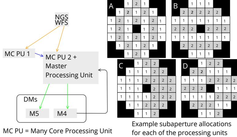
Figure 5. The architecture of the multi-node SCAO system setup as described in Section 2.3, this is an example for the ESO ELT. The WFS is multicast to the two processing units each of which process half of the total WFS subapertures, the master processing unit receives the partial DM vectors before combining them and delivering them to the DM.
