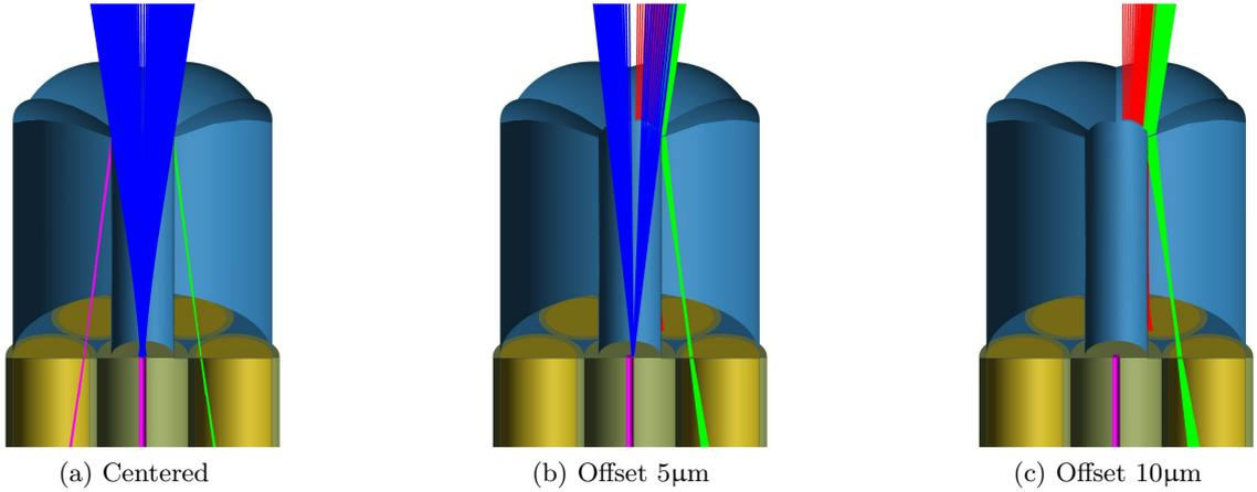
Figure 1. Modeled ray propagation through the micro-lens ring (MLR) for an incoming beam that is (a) aligned and offset by (b)  $5\mu\text{m}$  and (c)  $10\mu\text{m}$ , respectively. In the platescale of iLocator frontend (at  $1\mu\text{m}$ ), the diffraction limit  $1.22\lambda/D \sim 60\text{mas}$  corresponds to  $\sim 3.9\mu\text{m}$  offset. Please note that the number of rays propagating to the tip of the single-mode fiber (SMF) does not correspond to the coupling efficiency.
