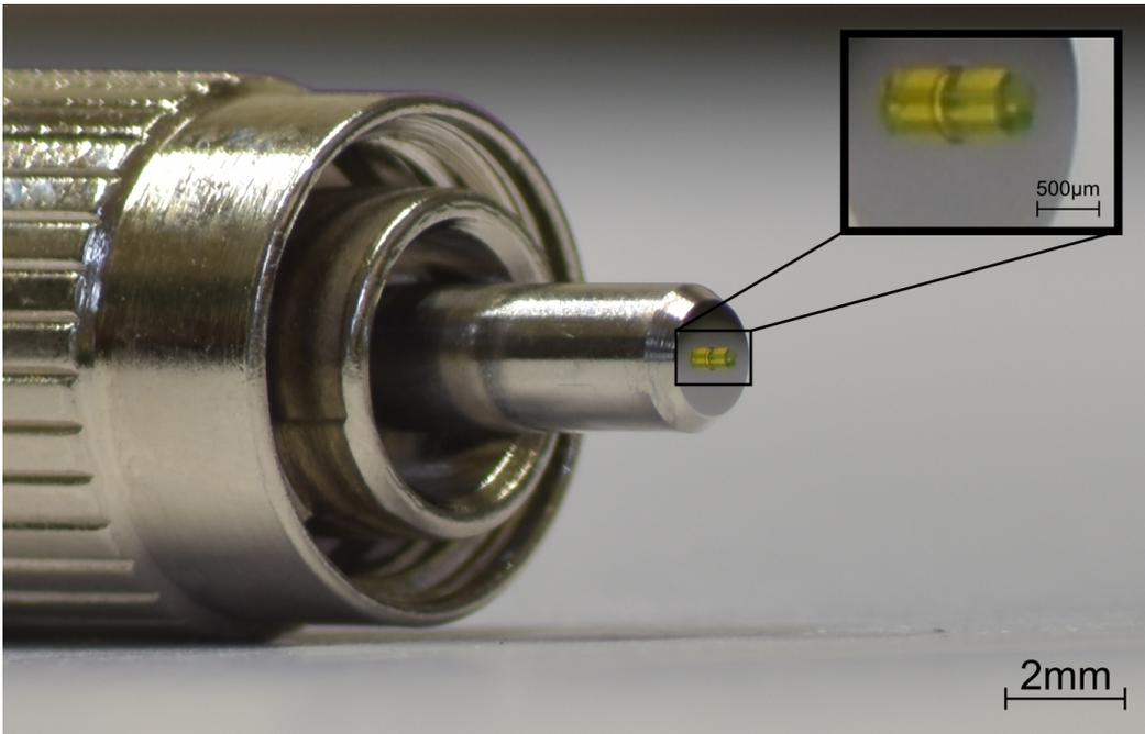
Figure 2. DSLR photograph of micro-lens ring (MLR). The lens stands around  $380\mu\text{m}$  tall and around  $400\mu\text{m}$  in diameter.
