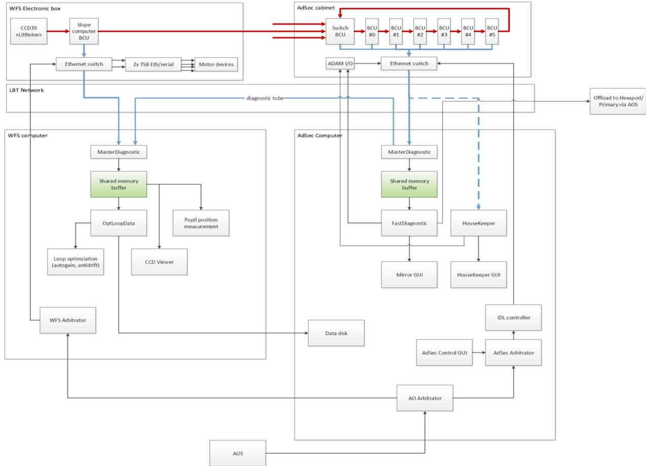
Figure 7. Optical Loop Diagnostic data transmission scheme.
