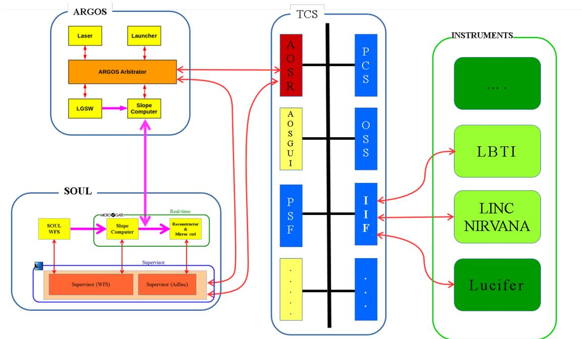
Figure 1. SOUL WFS Software interactions with the TCS.
