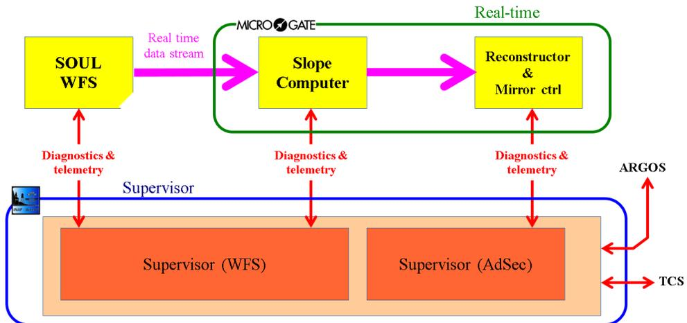
Figure 2. WFS and AdSec Hardware and Software mapping.
