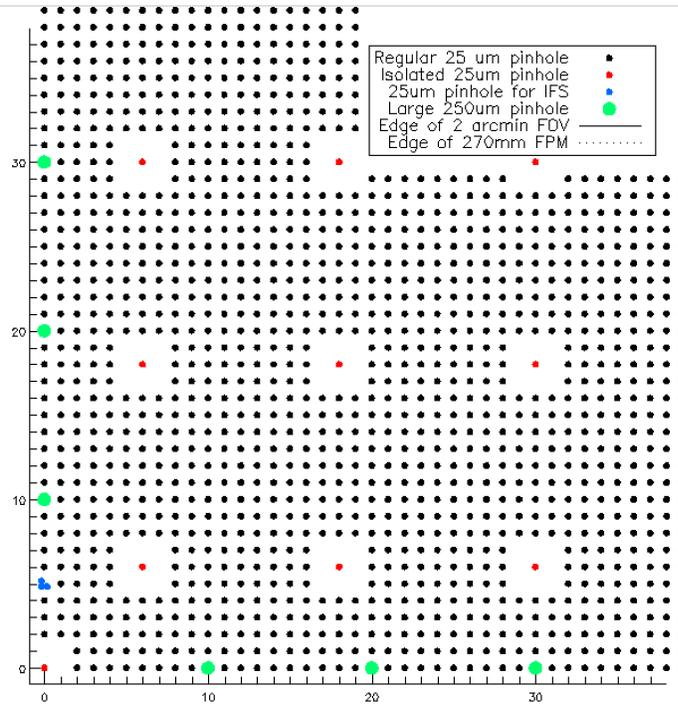
Figure 3: FPM layout in the central region (only one quarter shown)
