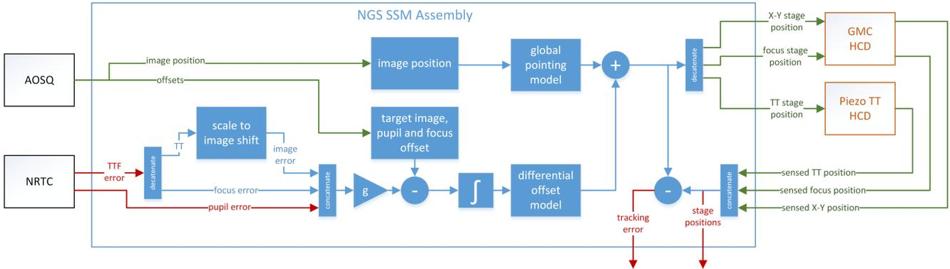
**Figure 6: NGS SSM Assembly block diagram during calibrations**
