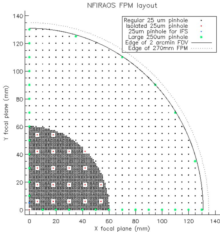
**Figure 2: FPM layout for the entire FOV (only one quarter shown)**
