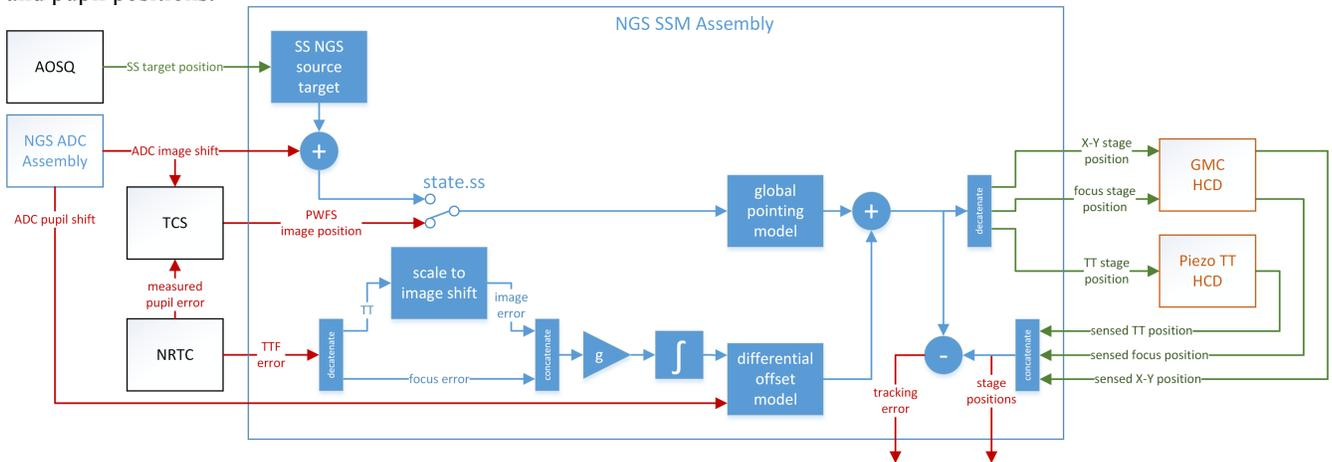
Figure 5: NGS SSM Assembly block diagram during operations
