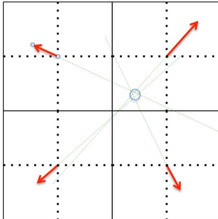
**Figure 7: Method to locate the position of an actuator based on slope measurements. The estimated location is a the intersection of the green dotted lines (blue circle), which are aligned with the slope vectors.**
