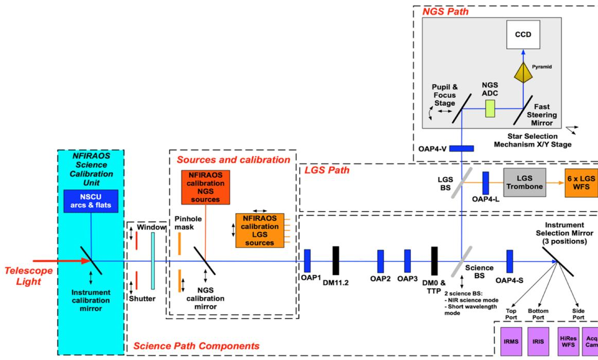
Figure 1: NFIRAOS top-level block diagram
