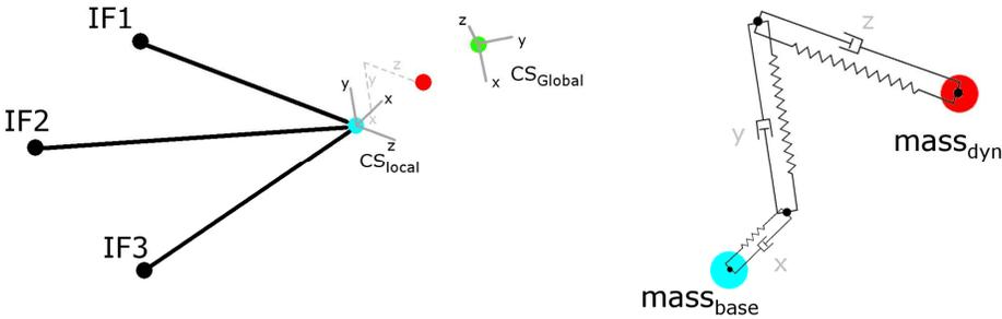
**Figure 7. Schematic representation of the subsystem mass decomposition and the addition of spring/damper elements.**
