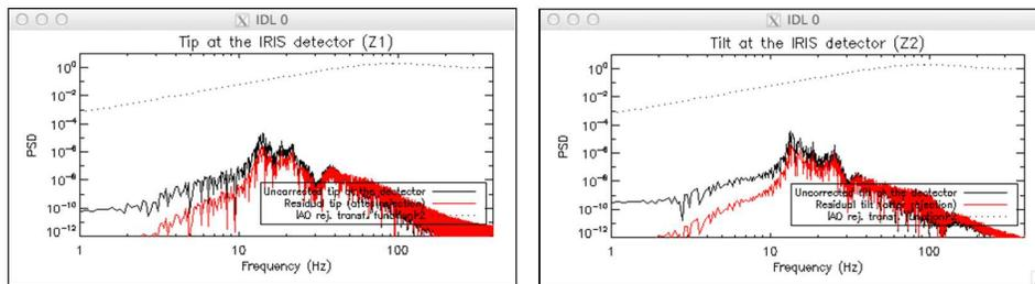
**Figure 9. PSD plots for the Tip and Tilt of the delivered image before and after the application of the AO rejection transfer function.**
