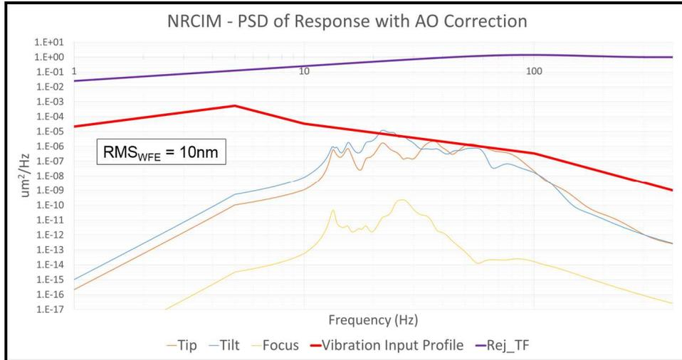
Figure 13. Dynamic optical performance in the presence of telescope vibration after convolution with the AO rejection transfer function.
