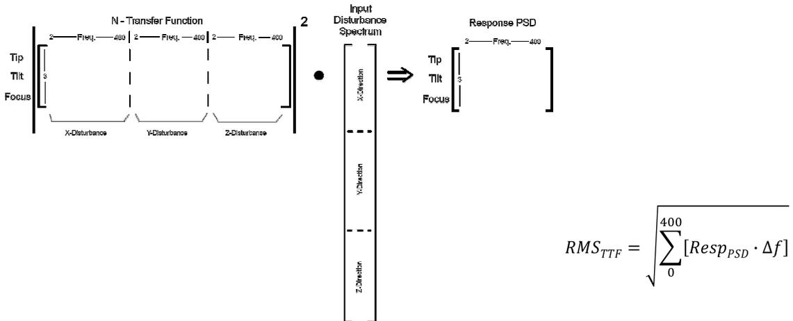
**Figure 12. Equation used to calculate the PSD response (and subsequent RMS) given an input disturbance PSD**
