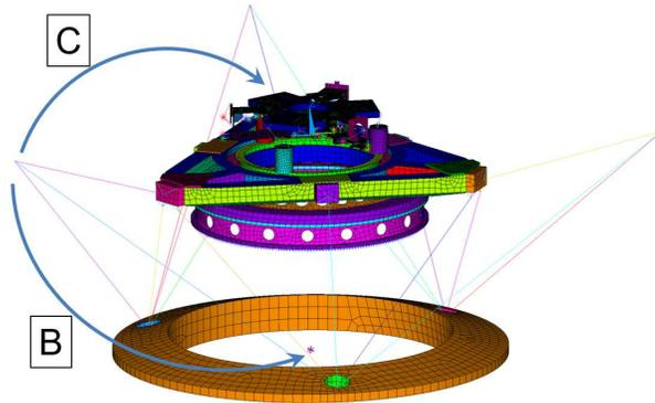
**Figure 15. FEM used to calculate the IRIS OIWFS imager transfer function.**
