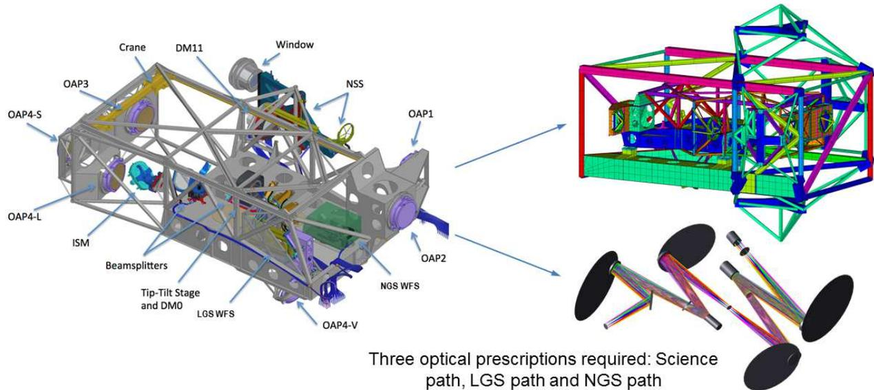
**Figure 3. NFIRAOS TABL and sub-system decomposition to the FEM and ZEMAX representations**
