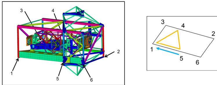
**Figure 4. NF-STR interface layout and association with TABL support points (yellow triangle).**
