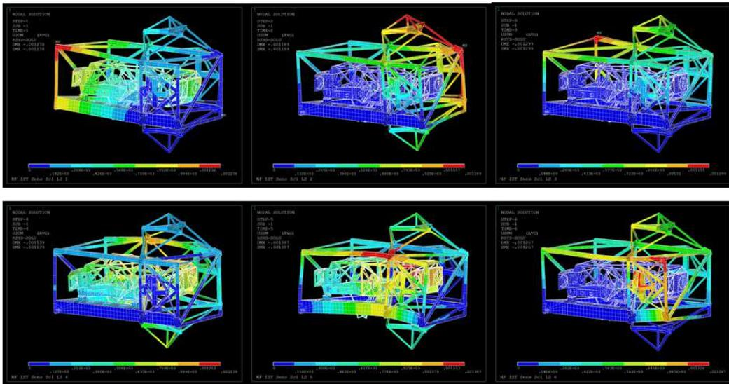
**Figure 5. Six deformed FEM results for the NF-STR interface sensitivity analysis.**
