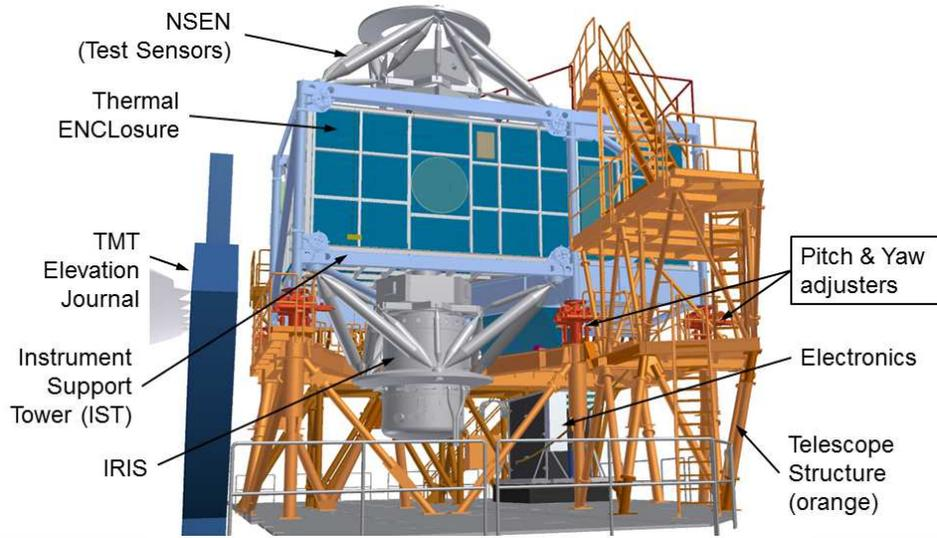
**Figure 2. Assembly view of NFIRAOS with instruments, mounted on the TMT telescope structure.**
