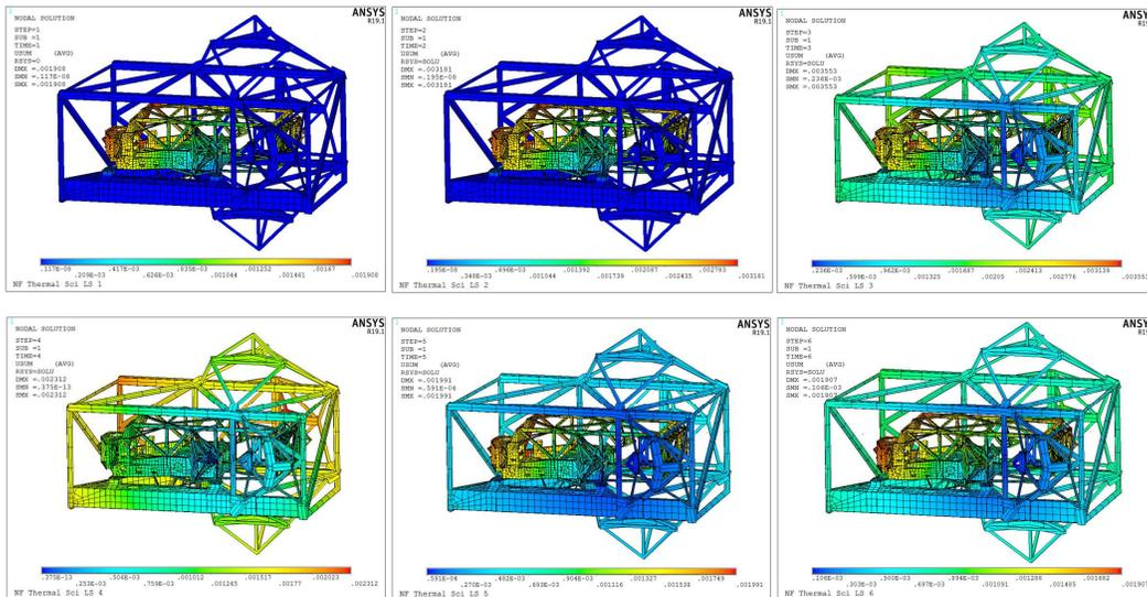
**Figure 6. FEA results of thermally-driven structural displacements.**
