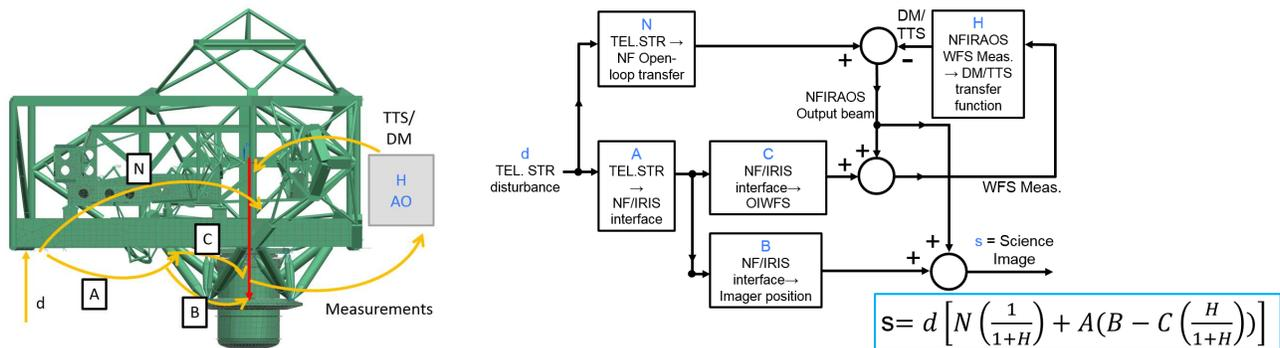
Figure 14. Graphical representation of the transfer functions required to combine NFIRAOS and IRIS (left) and the control flow chart for NFIRAOS and IRIS (right).
