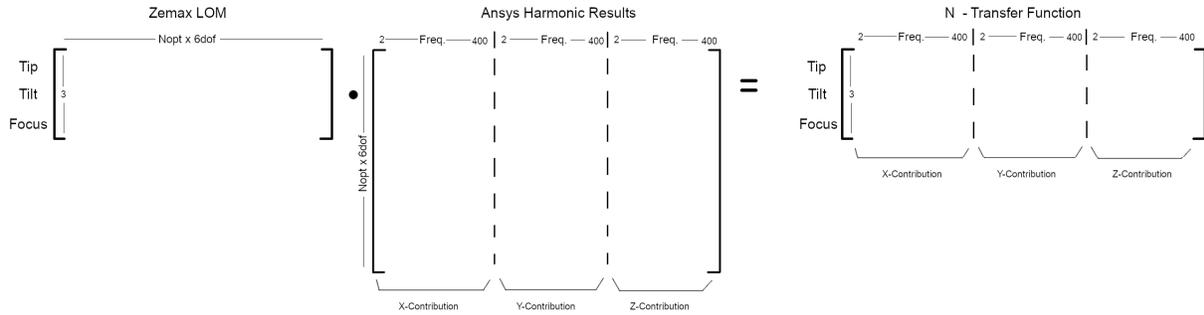
**Figure 11. Equation combining the LOM with the harmonic structural response to give the opto-mechanical transfer function.**
